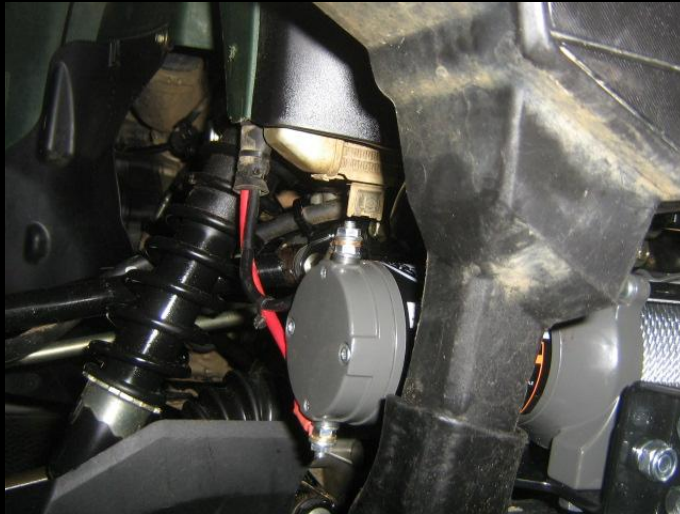
Note how the main power cable is tucked out of the way far enough for any but the gnarliest of terrain. Also pay attention to the quality locking hardware
